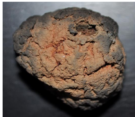
Figure 6. The calcinate sludge sample similar to baked clay.
