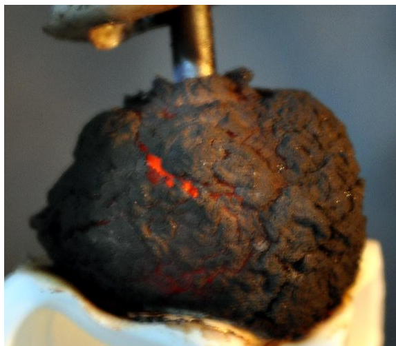
Figure 4. Sludge sample exposed to 1000W for 25 minute.
