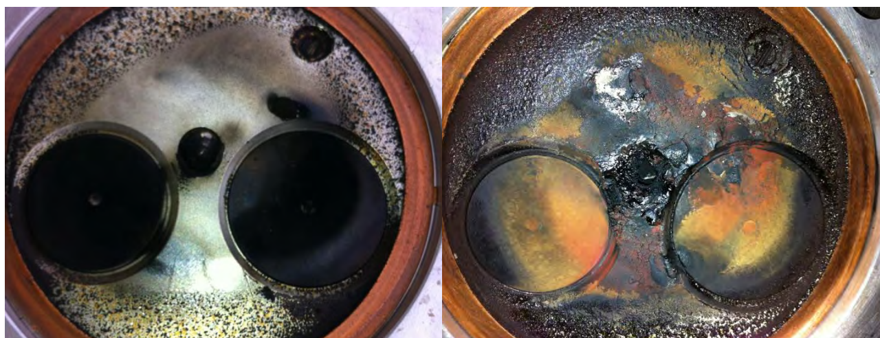
Figure 9. Carbon deposits on cylinderhead.
