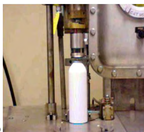
Figure 3. Pressure filling: a) Pressure fill button off. b) Single head pressure filler [8].
