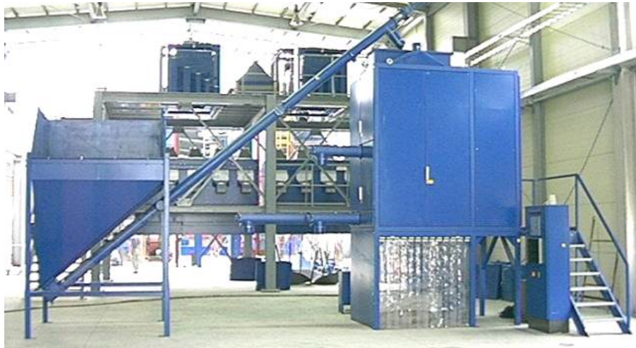
Figure 5. KWS corona-electrostatic separator, manufactured by Hamos, GmbH, Germany.
