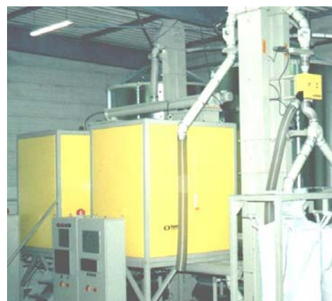
Figure 13. EKS tribo-electrostatic separator, manufactured by Hamos GmbH, Germany.
