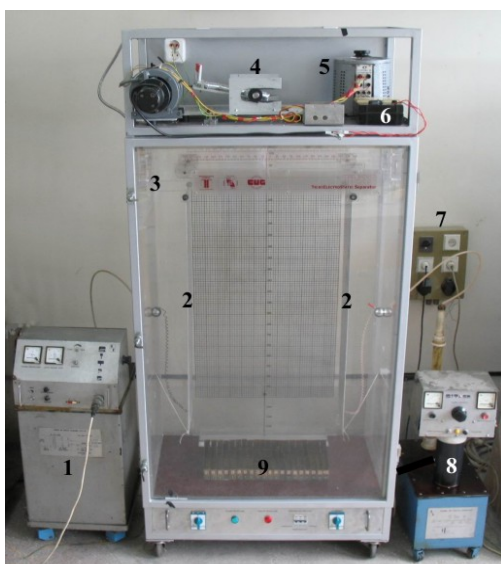
Figure 10. Free-fall tribo-vibro-electrostatic separator for mixed granular plastics [21]. 1: positive high-voltage supply; 2: plate electrodes; 3: separation chamber; 4: vibratory tribo-charger; 5: feed rate control; 6: frequency meter 7: control panel; 8: negative high-voltage supply; 9: collector.
