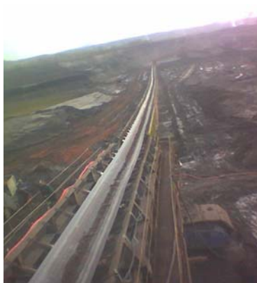
Figure 2. Belt conveyor in surface coal minning transport system.
