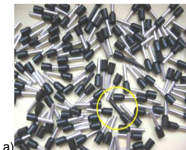
Figure 7. (a) Good and defect cable-end sleeves [19]; (b) Reject of the cable-end sleeves separation.
