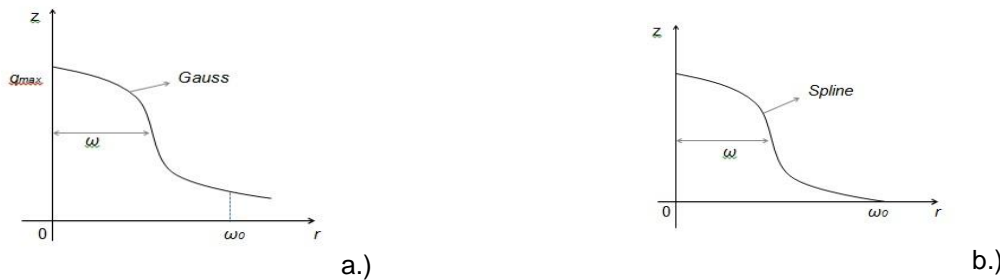
Figure 2. The geometrical image of the distribution of the heat flow for the Gauss model a). cubic spline b). regression.
