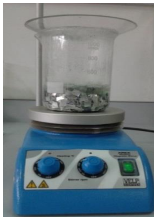
Figure 3. The process of coating removal from the aluminum surface.
