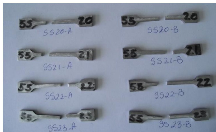
Figure 9. Broken specimens of T6 SSR material.
