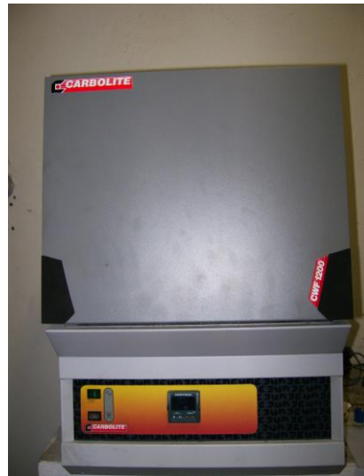
Figure 4. Carbolite electric furnace CWF 1200.
