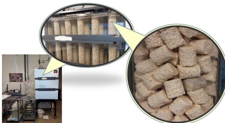
Figure 4. Description of a PBR reactor (Packed Bed Reactor).
