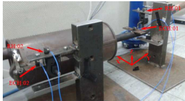
Figure 9. Exhaust line on rubber elements
