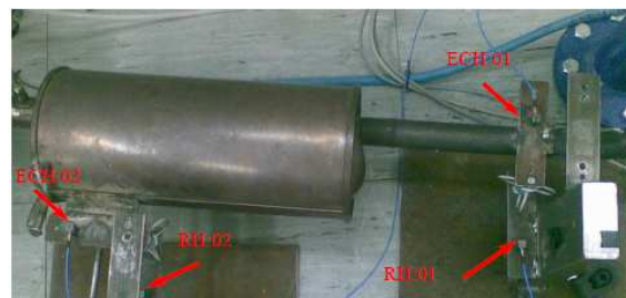
Figure 10. Exhaust line on wire rope elements
